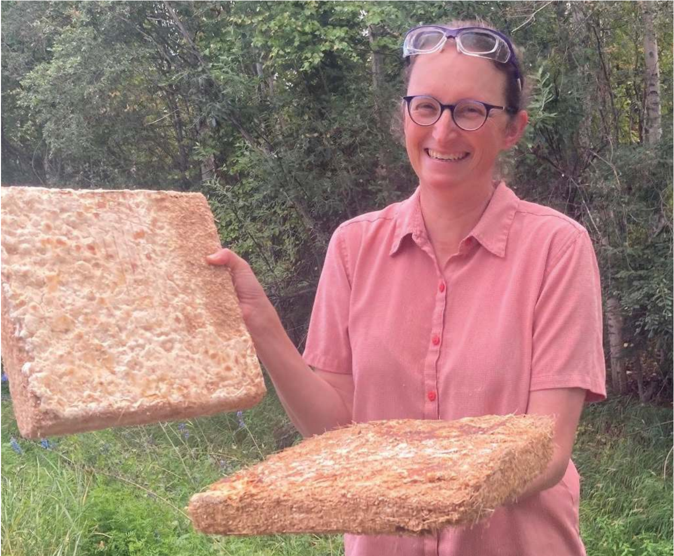
Engineer Robbin Garber Slaght holds prototype insulation panels made of wood fiber held together by a fungus species. Photo by Molly Rettig.
